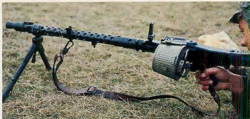
The world's first GPMG, the MG34, was the most elaborate machine gun ever manufactured. However, in combat it demonstrated itself to be overly sensitive to adverse environmental conditions, especially dust.
